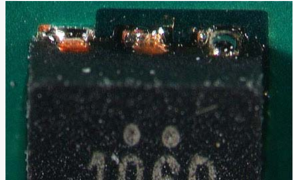
Figure 2. Exposed Copper on Package Edge, Solder Wetting after Reflow, from Singulation Process
