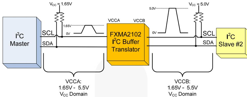
Figure 8. FXMA2102 I<sup>2</sup>C/SMBUS Translator Application
