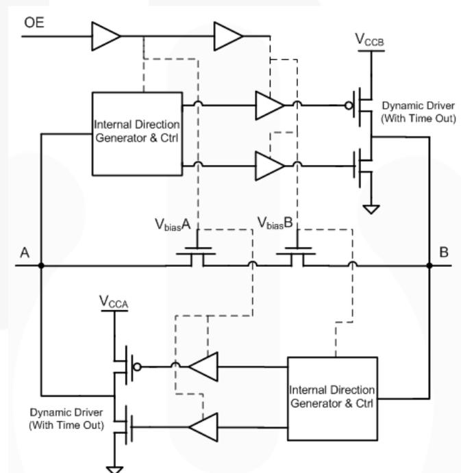
Figure 7. Hybrid Driver Block Diagram, One Channel
