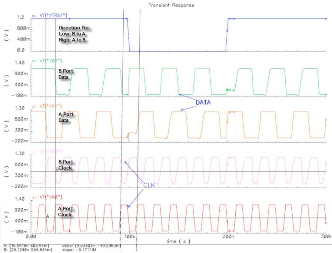
**Figure 11. Proprietary Chip-to-Chip Interface Direction Change Timing**
