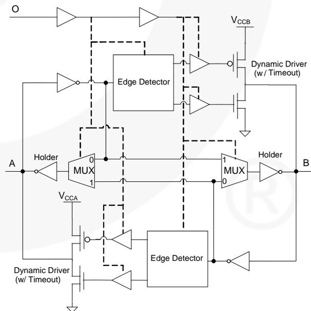
**Figure 5. Bus Hold Block Detailed Diagram, One Channel**
