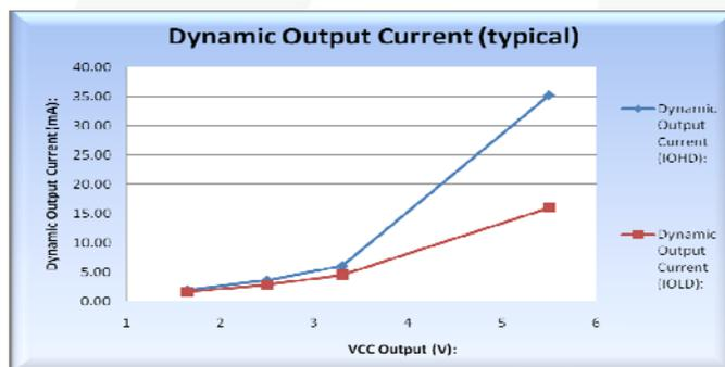
Figure 6. Dynamic Output Current of Auto-Direction Bus Hold
