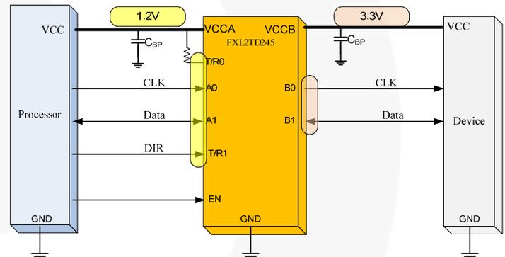
**Figure 10. Proprietary Chip-to-Chip 60 MHz Three-Wire Interface**
