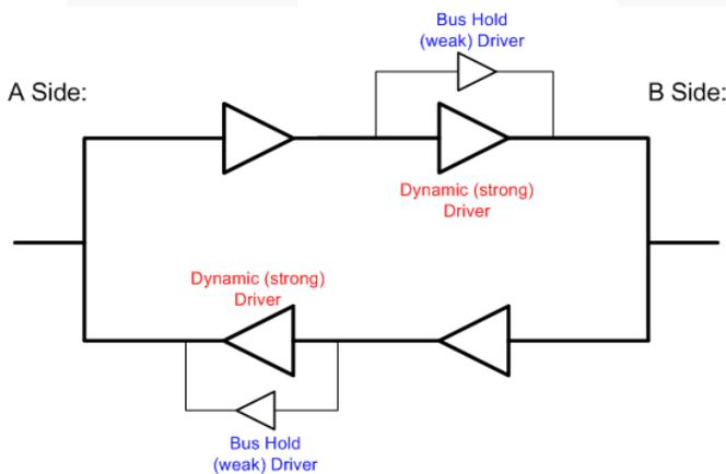
**Figure 4. Bus Hold Block Diagram, One Channel**
