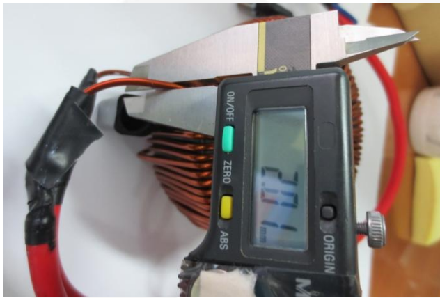
Figure 6. Copper Wire Width (2.01 mm)
