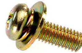
Figure 6. SEMS Screw (Size M3, Spring Washer 5.0Ø, Plain Washer 7.5Ø)
