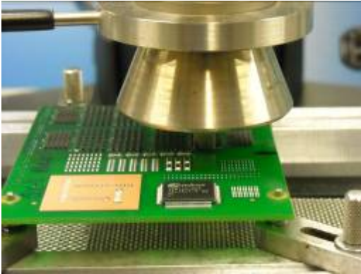
Figure 9. Hot Air Rework System Reflow
