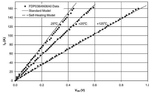
Figure 7. FDP038AN08A0 saturation voltage Conditions:  $V_{GS} = 10V$
