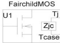
Figure 2 Self-heating MOSFET SPICE symbol
