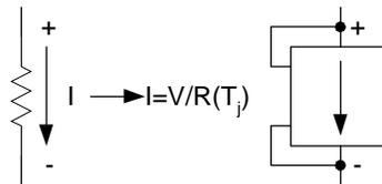
Figure 3. Implementing a voltage dependent ABM resistor model
