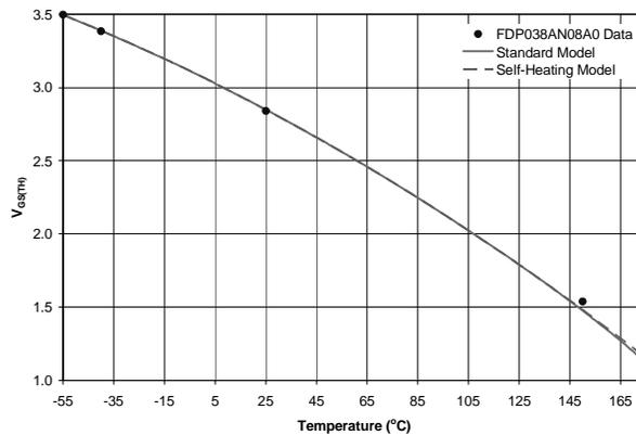
Figure 5. FDP038AN06A0 threshold voltage Conditions:  $I_D = 250\mu A$
