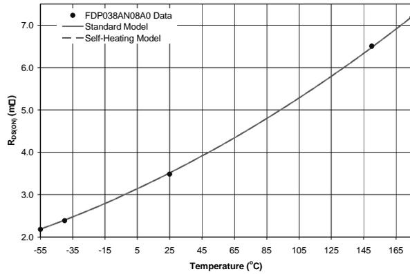
Figure 6. FDP038AN08A0  $r_{DS(ON)}$  Conditions:  $I_D = 80A$ ,  $V_{GS} = 10V$
