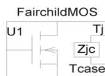
Figure 3. Self-heating MOSFET SPICE symbol
