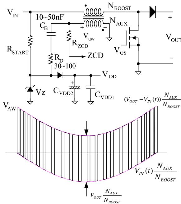
Figure 10.  $V_{DD}$  Supply Circuit using Auxiliary Winding
