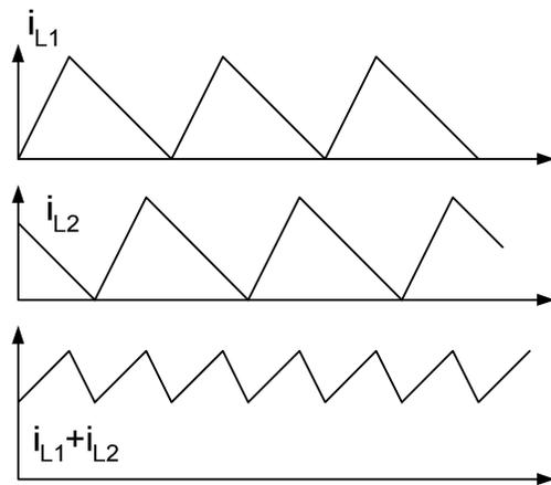
Figure 6. Interleaving Operation of BCM Boost PFC
