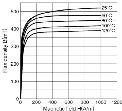
Figure 8. Typical B-H Curves of Ferrite Core
