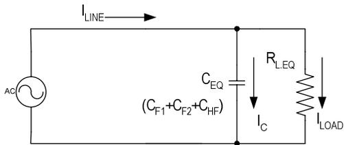
Figure 21. Equivalent Circuit of Line Filter Stage
