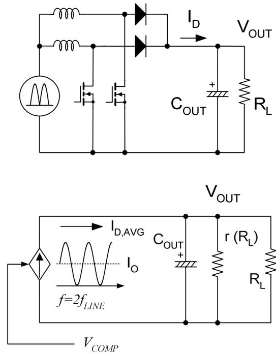
Figure 17. Small Signal Modeling of the Power Stage
