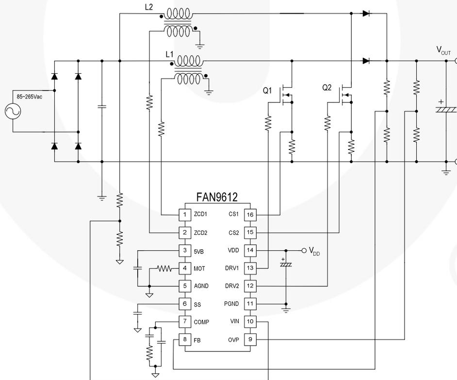
Figure 1. Typical Application Circuit of FAN9611 or FAN9612
