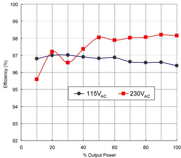
Figure 31. Measured Efficiency
