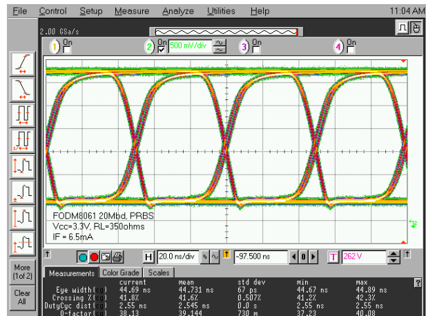
Figure 11. 20MBd Eye Diagram
