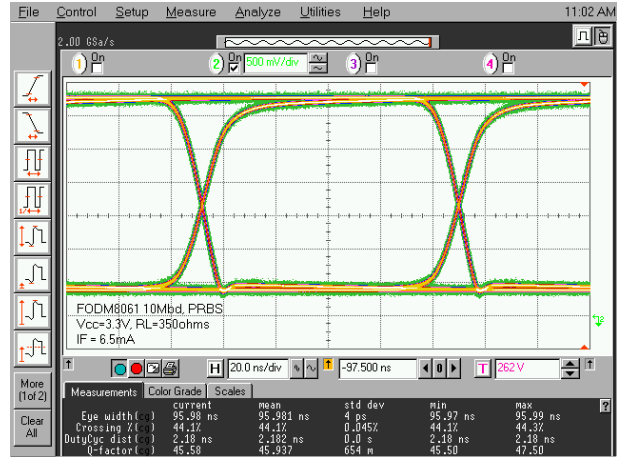
Figure 10. 10MBd Eye Diagram
