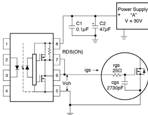
**Figure 12. FOD3120 – MOSFET Interface**
