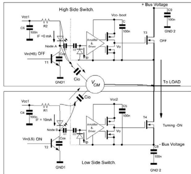
Figure 9. Low-Side ON, High-Side OFF, Negative CMT
