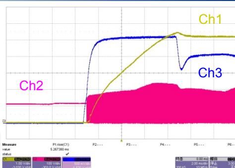
Figure 16. 85 V AC / 60 Hz at Max. Load (Ch 1: V O , Ch 2: V DS , Ch 3: V FB )
