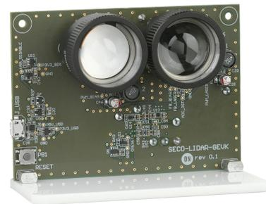
Figure 1. SECO-RANGEFINDER-GEVK
