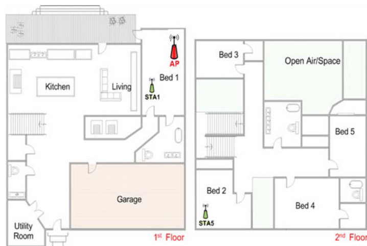
Figure 1. Example of Home Deployment with Two Set Top Boxes in a Typical Home
