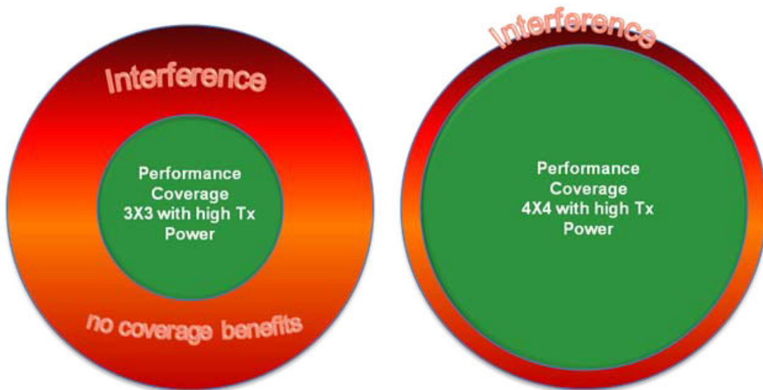
Figure 7. With High Tx Power, Higher order MIMO Provides Unparalleled Coverage
