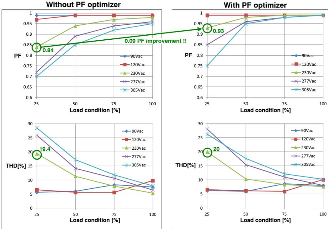
Figure 9. Power Factor & Total Harmonic Distortion Comparison
