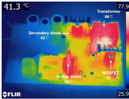
Figure 18.  $V_{IN} = 90 V_{AC}$
