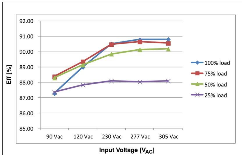
**Figure 11. Efficiency by Line Voltage & Load Condition Change**
