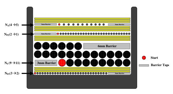
Figure 3. Transformer Winding Structure
