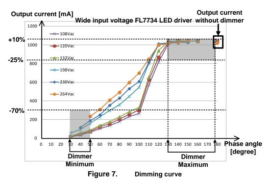
Figure 7 shows a dimming curve which is obtained by rotating the dimmer switch. Regardless of input line voltage  $\pm 10\%$  variation, LED current is constantly regulated from 180 to 130° dimmer phase angle .When the phase angle is below 130°, LED current decreases linearly according to internal dimming reference modulation.
