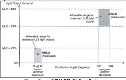
Figure 8. NEMA SSL-7A Specification
