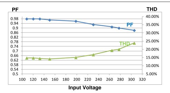
Figure 6. PF and THD data plotted against Line Variation – 40 V Nominal Load
