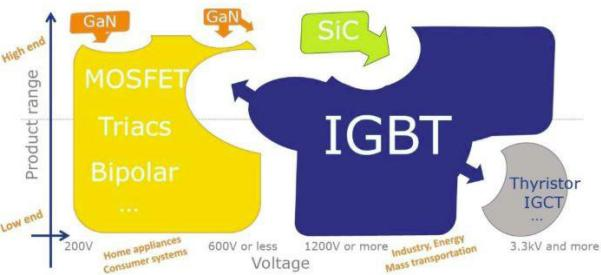
Figure 1. Power Switch Environment [1]
