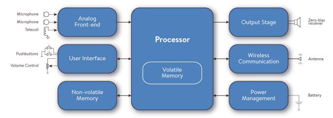
Figure 4. Main Functional Blocks Diagram
