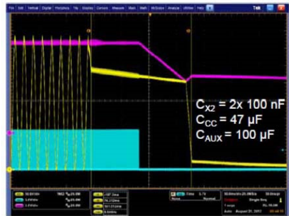
X2 Discharge at 265 VAC Ch. 1 (Yellow): BOX2 Voltage Ch. 2 (Blue): QR DRV Ch. 3 (Purple): V_{CC}
