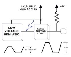
Simple NFET level translation techniques use the bidirectional nature of the FET and the low threshold voltage to "clamp" the lowside of the protection block to a reference voltage, such as the VDD of the low-voltage ASIC. Unexpected glitches and peaks that might normally destroy these integrated "tolerant" structures are easily absorbed by the relatively higher power external devices.
