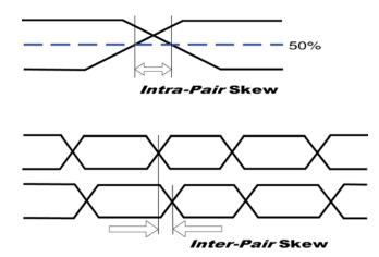
The HDMI Specification, Version 1.1 specifies "Intra-Pair Skew at Source Connector," at a maximum of 0.15\*Tbit, or less than about 90 ps @ 1.65 GHz. "Inter-Pair Skew at Source Connector" is a more "relaxed" 0.20\*Tpixel, or less than about 1.2 ns @ 165 MHz.
