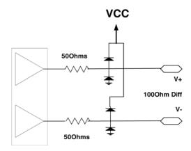
The channel capacitance of the reverse biased ESD clamp diodes and the parasitic series inductance of the package leads and bond wires (shown below) create a lumped resonant LC tank circuit that creates a low impedance shunt at the natural self-resonance frequency of the device.
