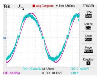
Figure 2. CrM Flyback Input Waveform
