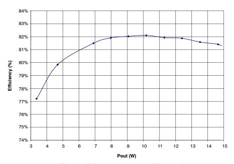
Figure 4. Efficiency versus load (Vin = 115 Vac)
