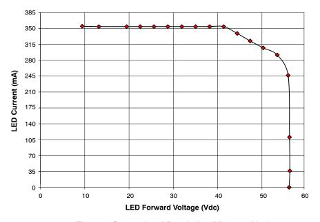
Figure 5. Current Load Regulation (Vin = 115 Vac)
