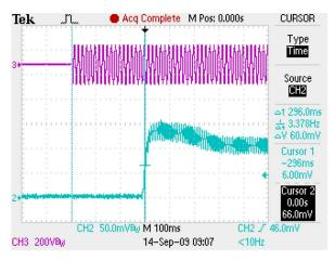
Figure 7. Startup Time (Vin = 115 Vac, 12 LED load)
