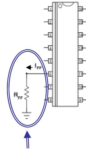
Pin 6 pins out a voltage proportional to the power. The  $I_{FF}$  current is clamped to  $105 \mu A$  and used to charge and discharge the oscillator capacitor
