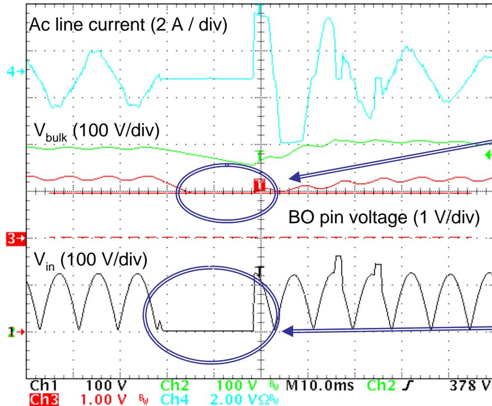
For the blanking time, the BO pin voltage is maintained around the BO threshold not to delay the circuit restart when the line has recovered
