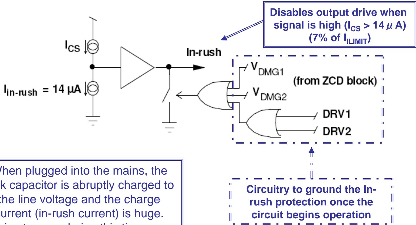
When plugged into the mains, the bulk capacitor is abruptly charged to the line voltage and the charge current (in-rush current) is huge. Drive turn-on during this time can damage the MOSFETs.
