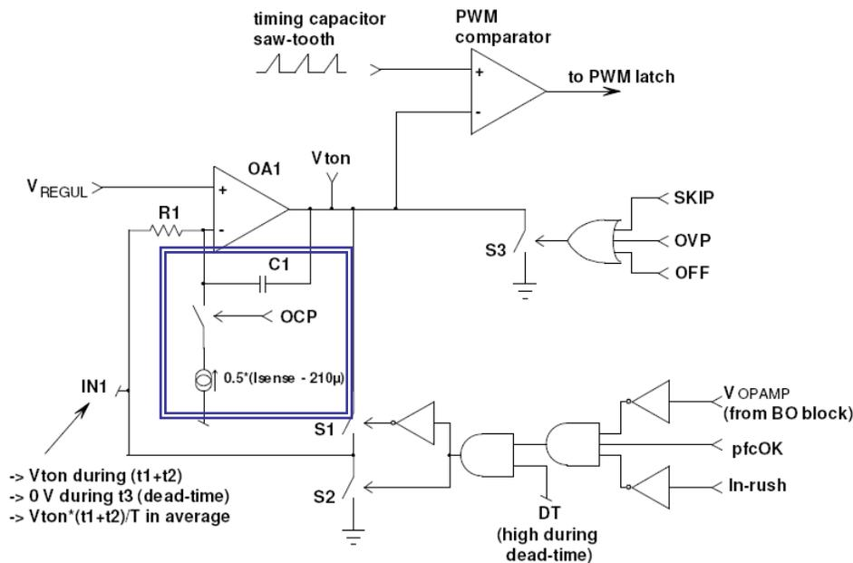
When  $I_{CS} > 210 \mu A$ , the OCP switch closes and a current equal to  $0.5 \cdot (I_{CS} - 210 \mu A)$  is injected into the negative input of the  $V_{TON}$  processing opamp
