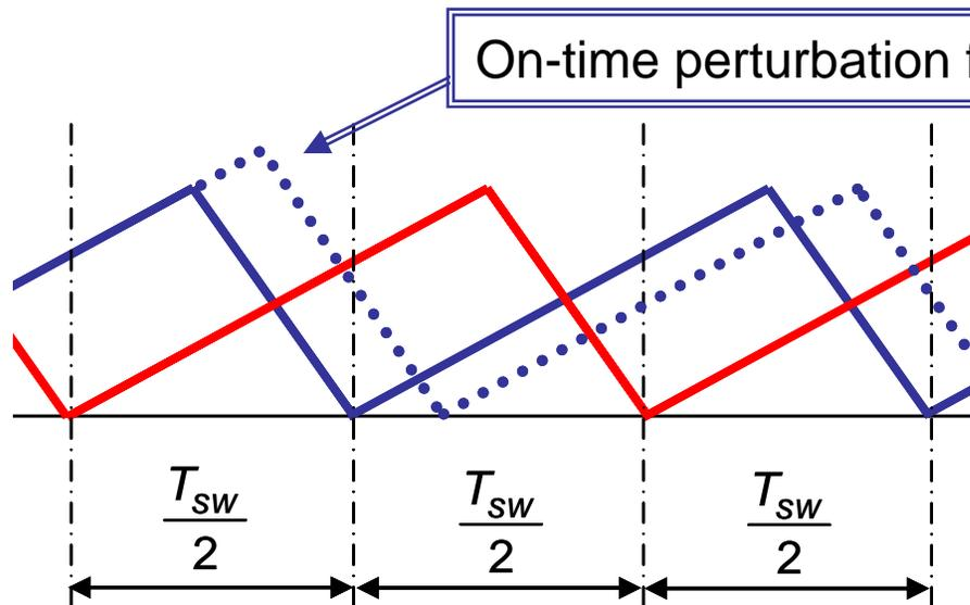
CrM operation is maintained but a perturbation of the on-time may degrade the  $180^\circ$  phase shift
