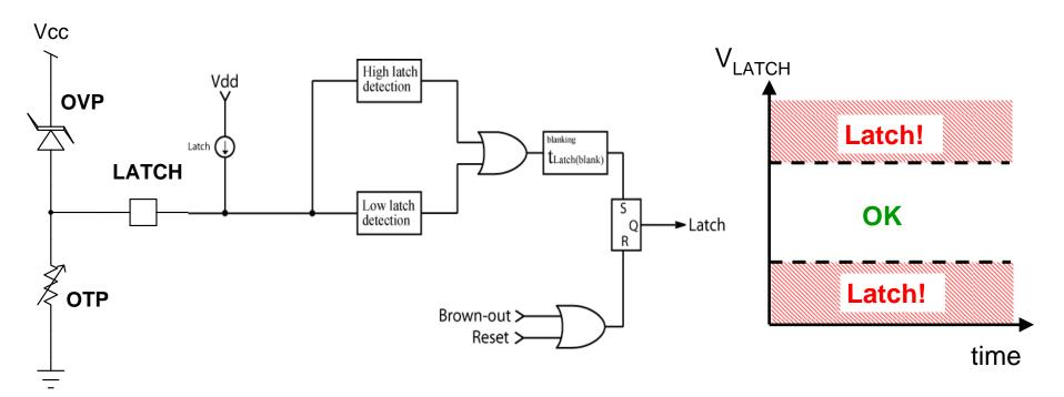
An NTC thermistor can be directly connected to the IC
