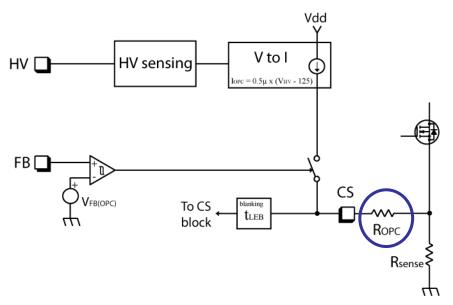
Need to compensate for the effect of the propagation delay
