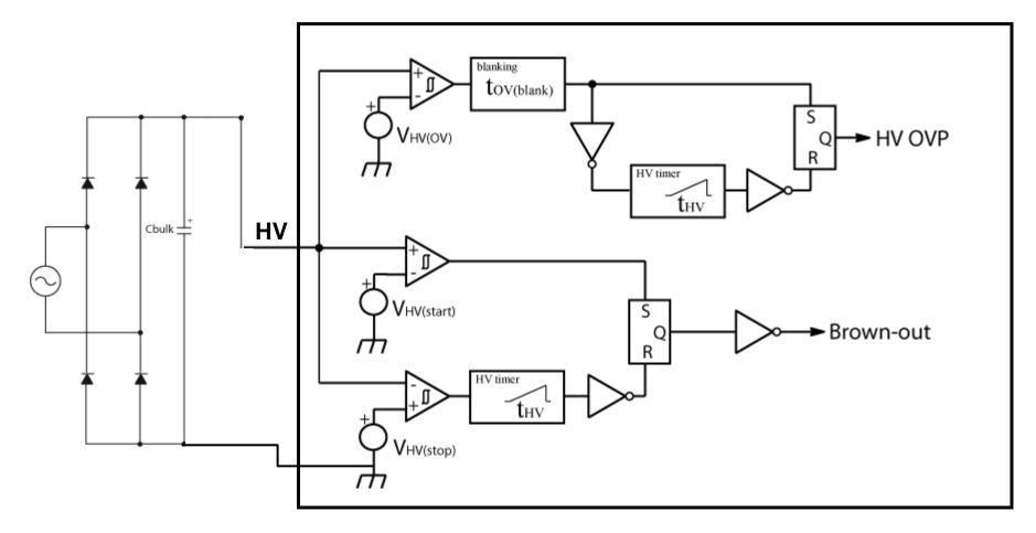
Detection independent of Ripple on HV pin
