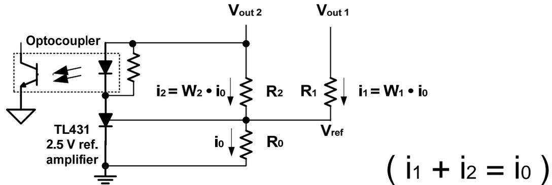
$$V_{out1} - V_{ref} = i_1 R_1$$
