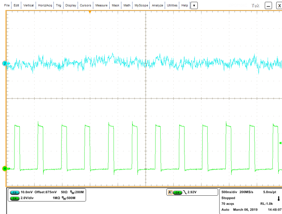
Figure 17: Ripple when the switcher is in forced PPWM mode at 5A load. Switching frequency is not constant therefore ripple is not shaped consistently. CH2 is output voltage and CH4 is SWN.
