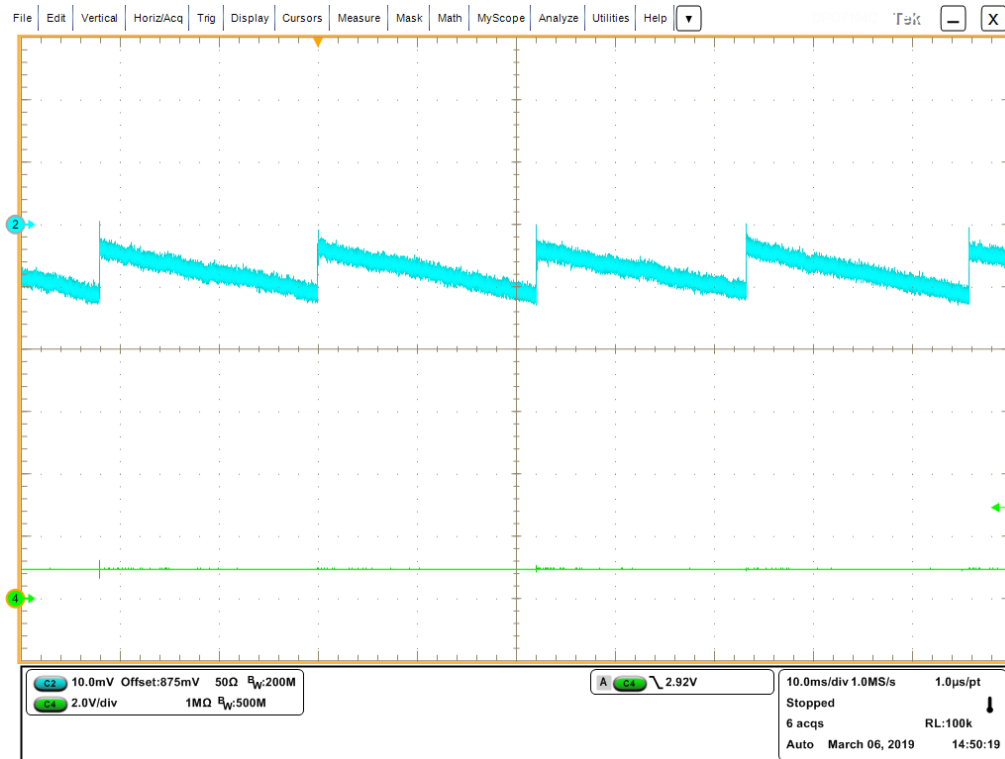
Figure 19: Ripple when switcher is in Auto mode and 0A. This is zoomed out from previous figure.
