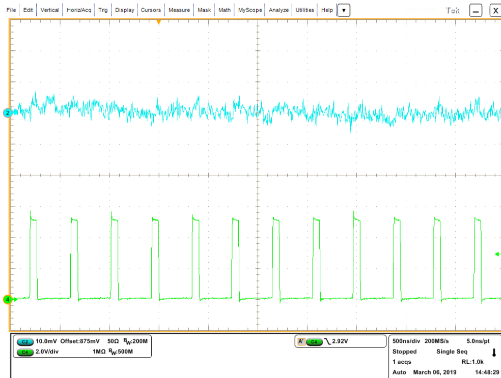
Figure 16: Ripple when the switcher is in forced PPWM mode at 0A load. Switching frequency is not constant therefore ripple is not shaped consistently. CH2 is output voltage and CH4 is SWN.
