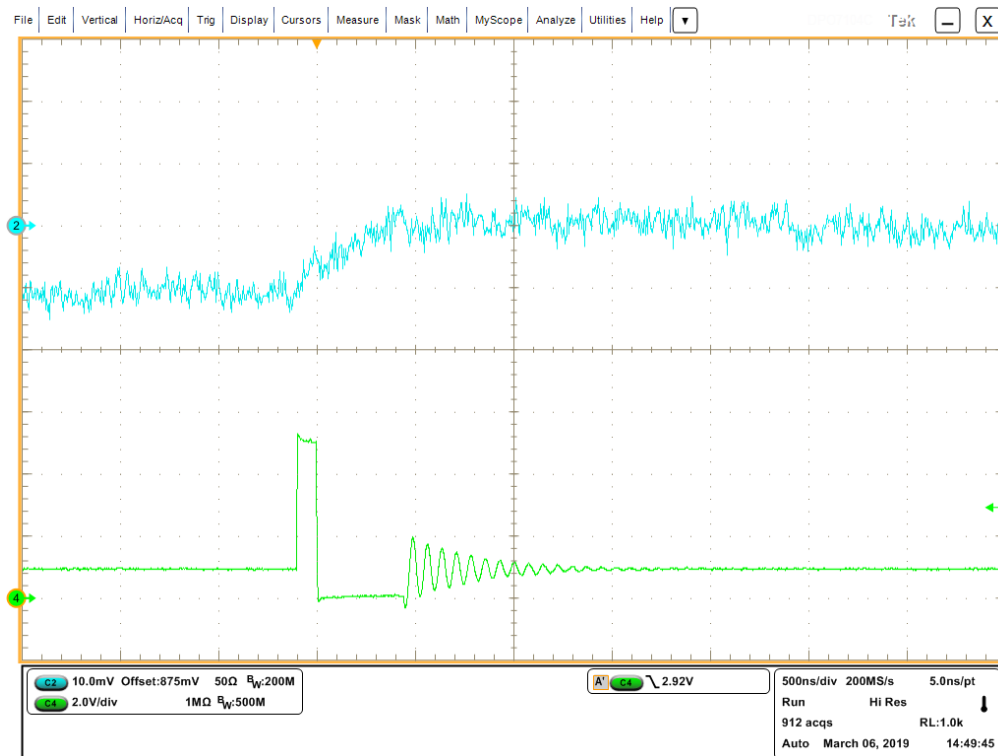
Figure 18: Ripple when the switcher is in Auto mode at 0A. CH2 is output voltage and CH4 is SWN.
