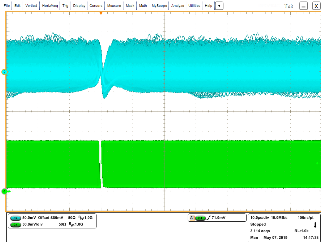
Figure 32: Transient sweep from 1kHz to 1MHz and a load step from 0.5A to 5A.
