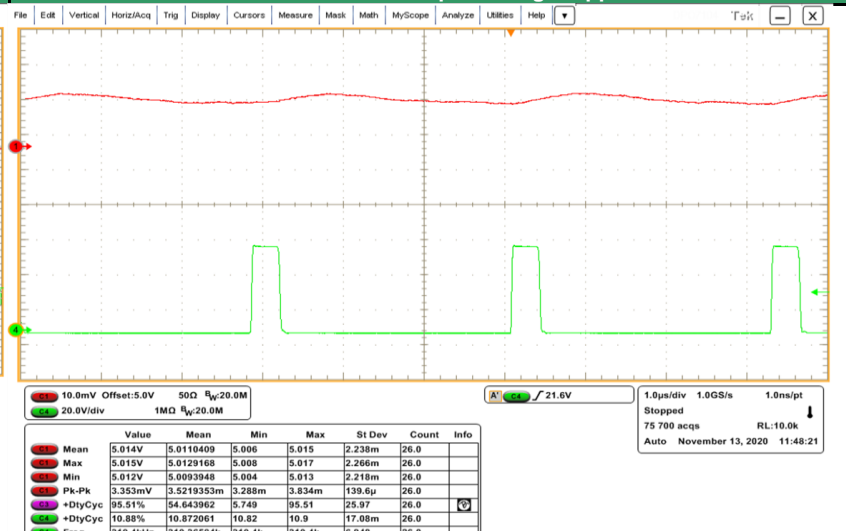
5Vout at 48Vin - TC2 Output Voltage Ripple at 6A
