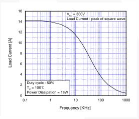
Fig 4. Load Current vs. Frequency
