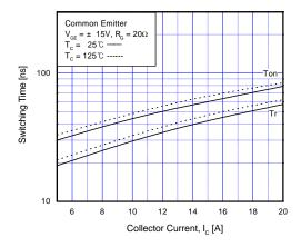
Fig 11. Turn-On Characteristics vs. Collector Current
