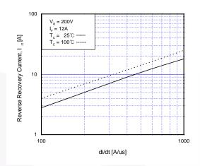
Fig 19. Reverse Recovery Current
