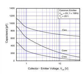
Fig 7. Capacitance Characteristics
