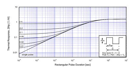
Fig 17. Transient Thermal Impedance of IGBT
