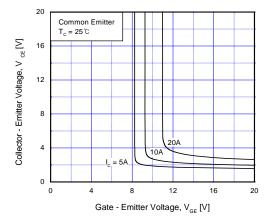
Fig 5. Saturation Voltage vs. V<sub>GE</sub>
