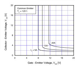
Fig 6. Saturation Voltage vs. V<sub>GE</sub>
