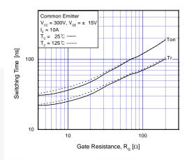
Fig 8. Turn-On Characteristics vs.
