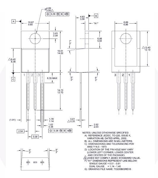
Figure 22. TO-220 3L - TO-220, MOLDED, 3LEAD, JEDEC VARIATION AB
