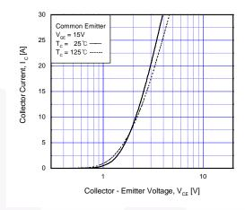
Fig 2. Typical Saturation Voltage Characteristics
