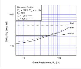
Fig 10. Switching Loss vs. Gate Resistance
