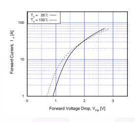
Fig 18. Forward Characteristics
