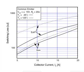
Fig 13. Switching Loss vs. Collector Current
