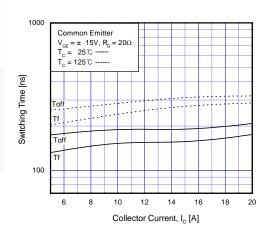
Fig 12. Turn-Off Characteristics vs. Collector Current
