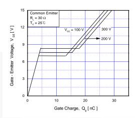
Fig 14. Gate Charge Characteristics
