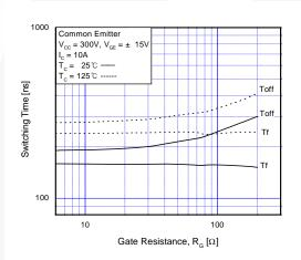
Fig 9. Turn-Off Characteristics vs.
