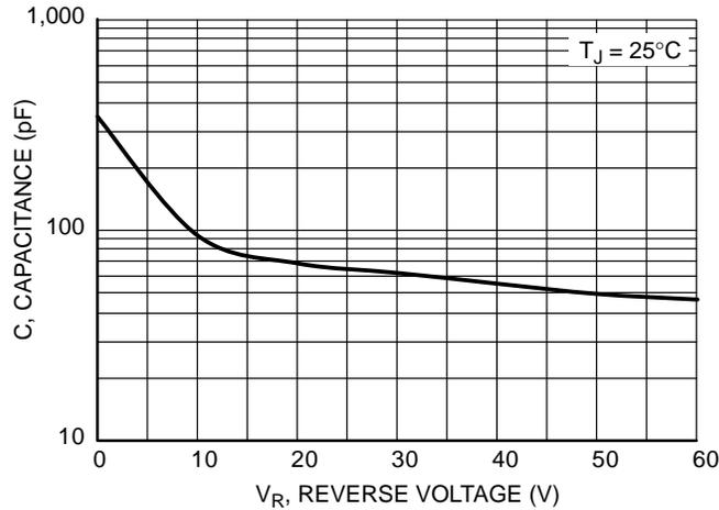
Figure 5. Typical Capacitance
