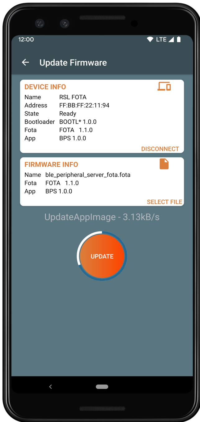
Figure 25. RSL FOTA Mobile Application: Updating Firmware
