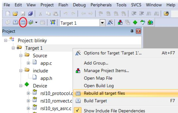
Figure 22. Starting to Build a Project in the Keil μVision IDE
