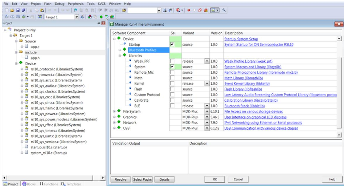
Figure 21. RTE Configuration for the Blinky Example Project in the Keil μVision IDE
