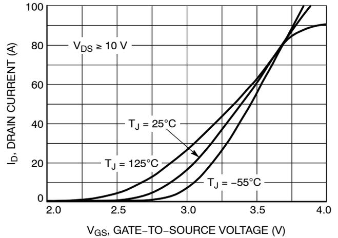
Figure 2. Transfer Characteristics
