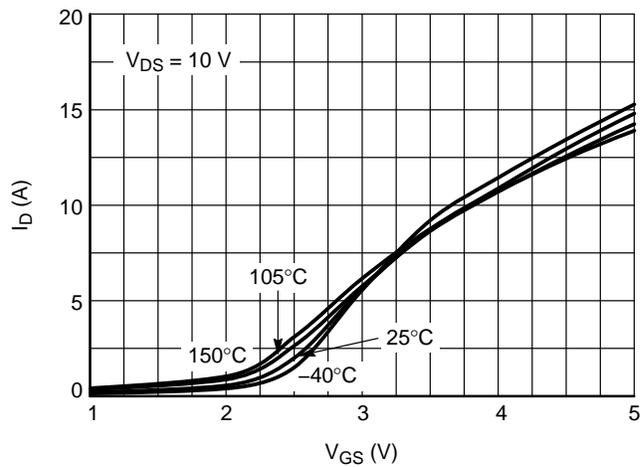
Figure 8. Transfer Characteristics
