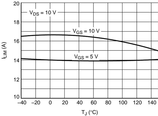
Figure 13. Current Limit vs. Junction Temperature
