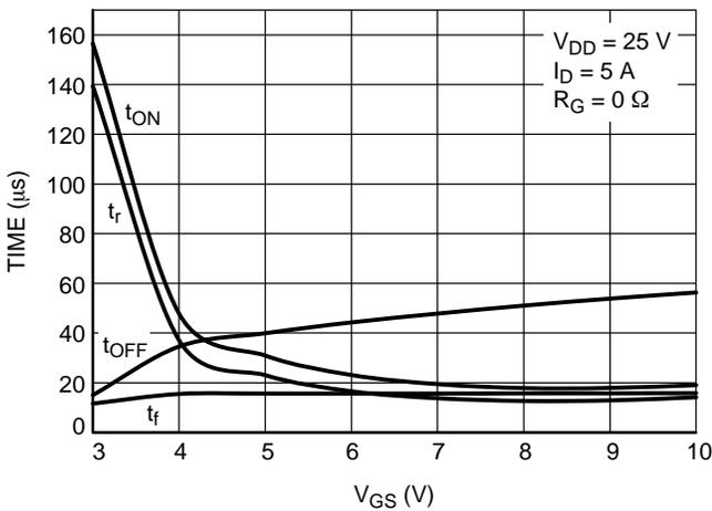
Figure 17. Resistive Load Switching Time vs. Gate-Source Voltage
