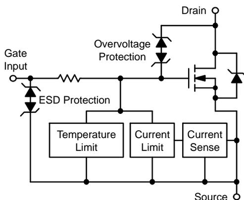
Figure 1. Block Diagram
