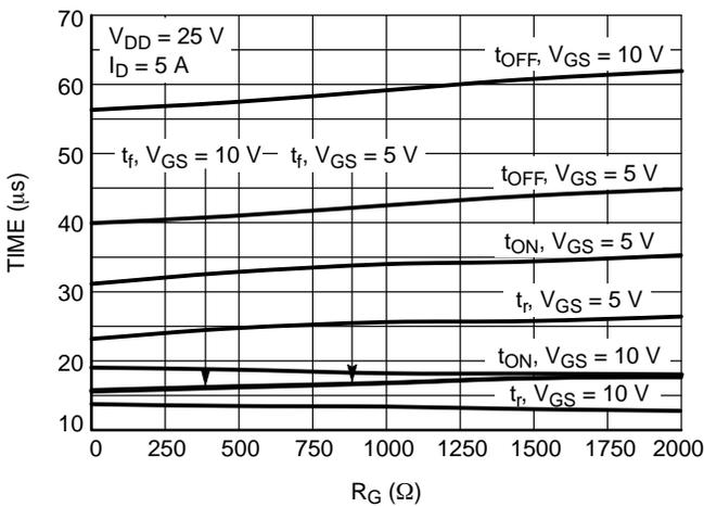
Figure 19. Resistive Load Switching Time vs. Gate Resistance
