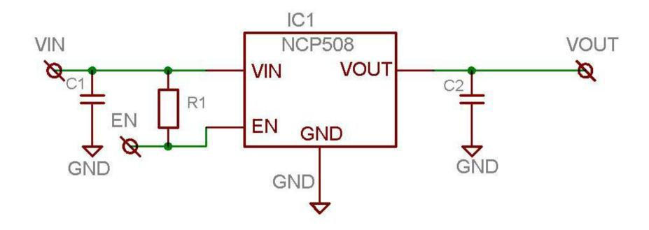
NCP508, 50mA, Fixed Output Voltage LDO Schematic View
