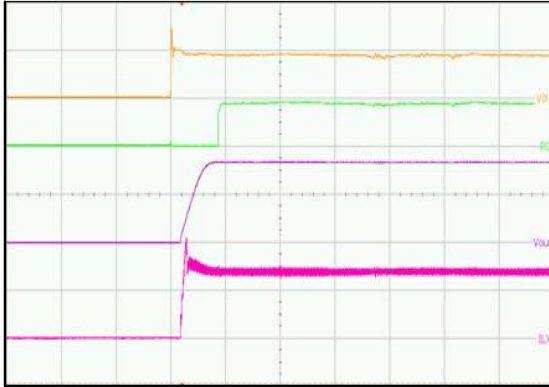
(VIN = 5 V, VOUT = 1.8 V, IOU = 3 A) Upper Trace: Input Voltage, 5 V / div Second Trace: Power Good Pin Voltage, 5 V / div Third Trace: Output Voltage, 2 V / div Lower Trace: Inductor Current, 2 A / div Time = 1 ms / div
