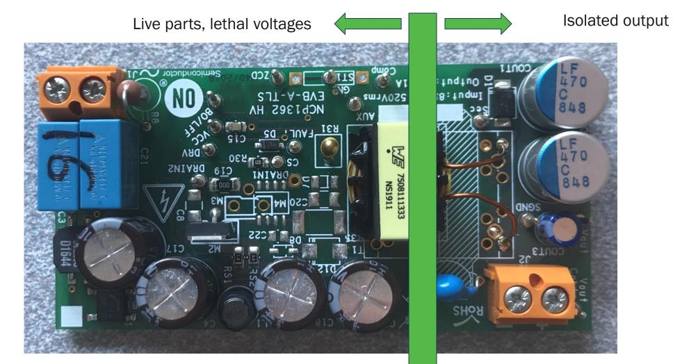
Input voltage from 85 V rms to 500 V rms
