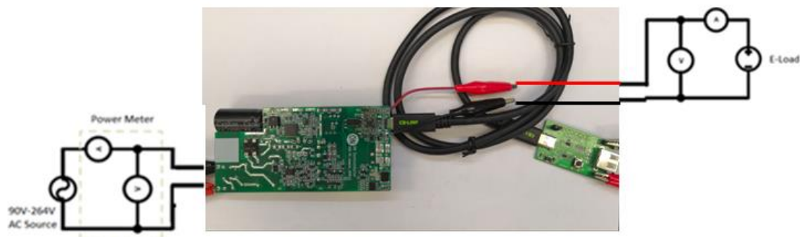
Figure 1: PD Test Setup for 90W PD/QC Demoboard
