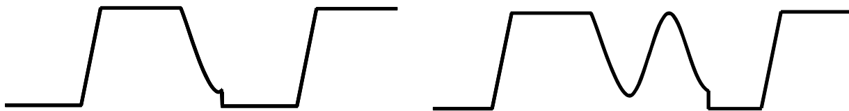
Figure 63. Full-load Operation – Quasi-resonant Mode in low line (left), turn on at valley 2 when in high line (right)
