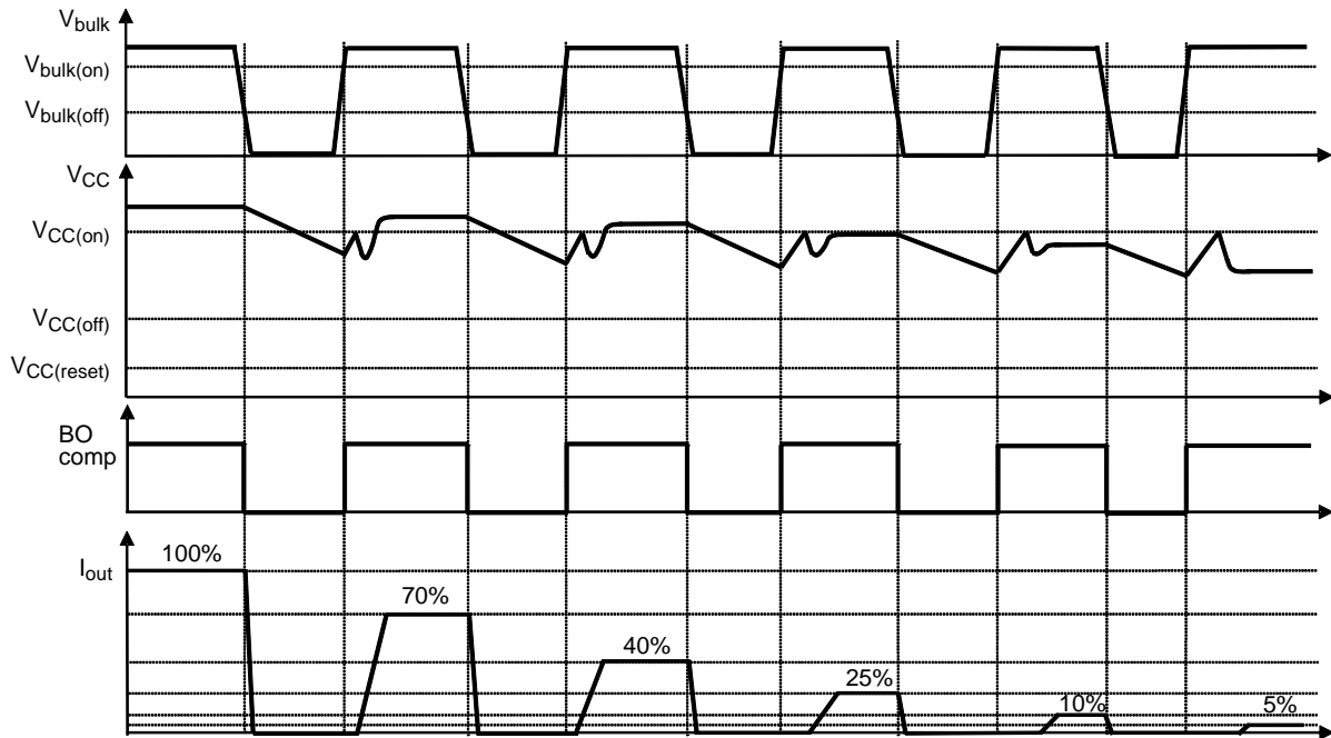
Figure 63. Step Dimming Chronograms
