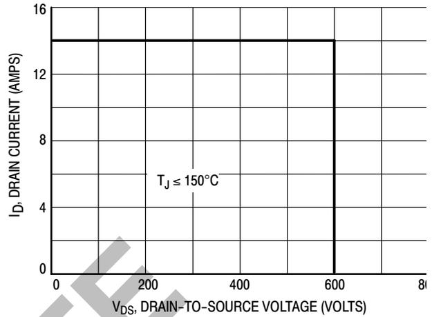
Figure 8. Maximum Rated Switching Safe Operating Area
