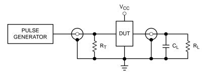
$C_L=50$  pF at  $V_{CC}=3.3\pm0.3$  V or equivalent (includes jig and probe capacitance)  $C_L=30$  pF at  $V_{CC}=2.5\pm0.2$  V or equivalent (includes jig and probe capacitance)  $R_L=R_1=500~\Omega$  or equivalent
