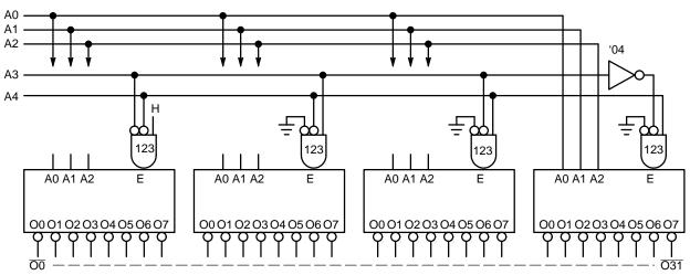
Figure 3. Expansion to 1-of-32 Decoding
