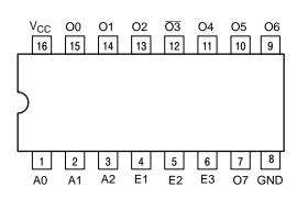
Figure 1. Pinout: 16-Lead (Top View)
