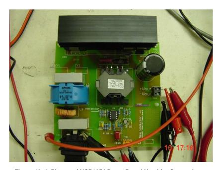
Figure 10-1. Picture of NCP1654 Demo Board Used for Comparisons
