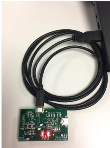
Figure 1 – FUSB302 EVB connected to PC
