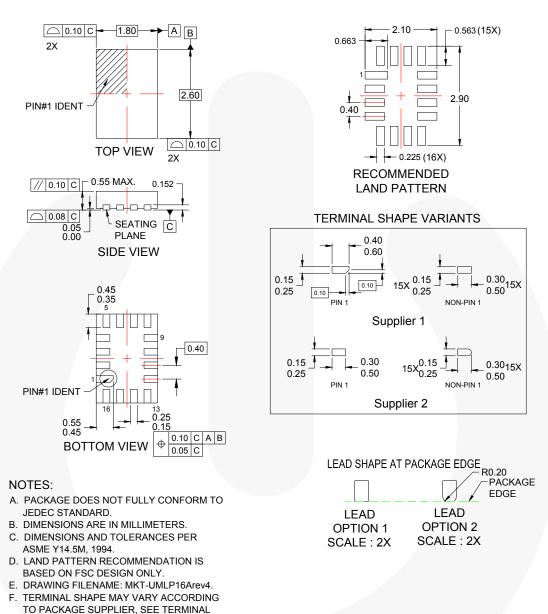
Figure 20. 16-Pin Ultrathin Molded Leadless Package (UMLP)
