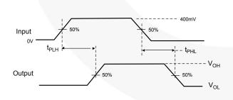
Figure 12. Propagation Delay (t<sub>R</sub>t<sub>F</sub> - 500ps)
