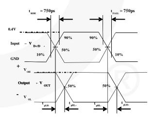
Figure 13. Skew Test Waveforms  $t_{SK(P)} = |t_{PLH-} - t_{PHL-}|$  or  $|t_{PLH+} - t_{PHL+}|$
