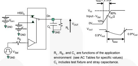
Figure 14. Break-Before-Make Interval Timing
