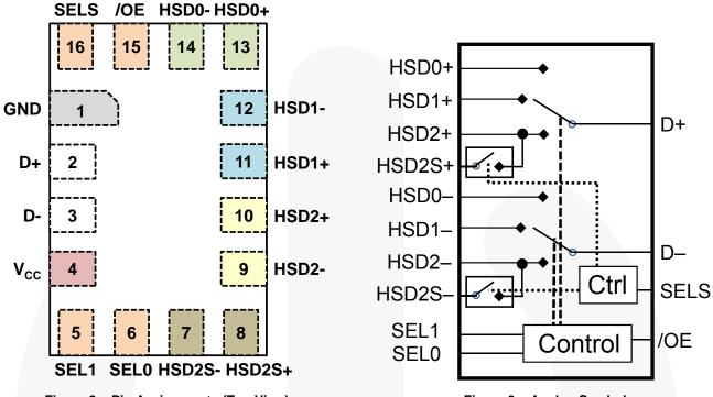
Figure 2. Pin Assignments (Top View)
