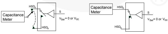
Figure 18. Channel Off Capacitance
