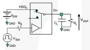
$R_L$ ,  $R_S$ , and  $C_L$  are functions of the application environment (see AC Tables for specific values)  $C_L$  includes test fixture and stray capacitance.
