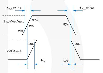
Figure 11. Turn-On / Turn-Off Waveforms
