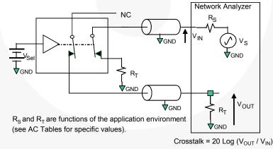
Figure 17. Non-Adjacent Channel-to-Channel Crosstalk
