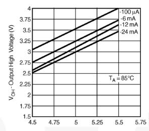
Figure 5. Output Voltage vs. Supply Voltage, V<sub>IN</sub> = V<sub>CC</sub>, T<sub>A</sub> = 85°C
