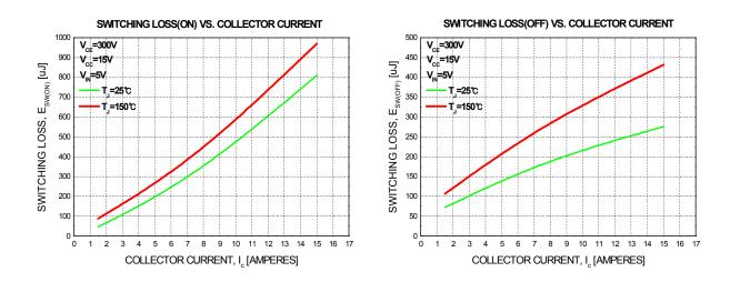
Figure 5. Switching Loss Characteristics
