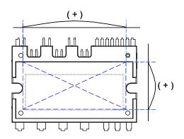
Figure 7. Flatness Measurement Position
