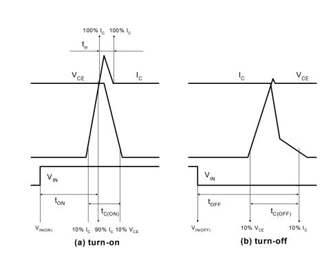
Figure 4. Switching Time Definition
