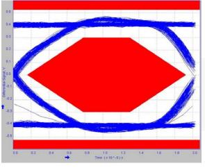
Figure 6. UART (TxD\_HOST/RxD\_HOST) High-Speed Eye Diagram
