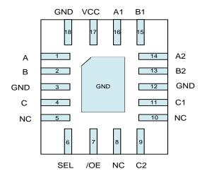
Figure 3. Pin Assignment(Top Through View)
