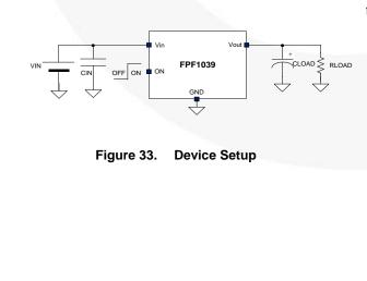
At maximum operational voltage ( $V_{IN}$ =5.5 V), device inrush current might be higher than expected. Spike current should be taken into account if  $V_{IN}$ >5 V and the output capacitor is much larger than the input capacitor. Input current can be calculated as:
