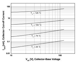
Figure 5. Collector-Base Cutoff Current
