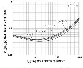
Figure 2. Collector-Emitter Saturation Voltage
