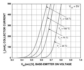
Figure 4. Base-Emitter On Voltage
