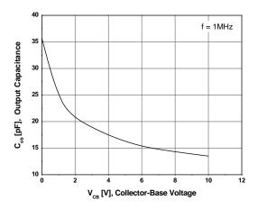
Figure 7. Output Capacitance
