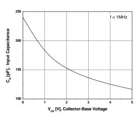
Figure 8. Input Capacitance
