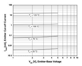
Figure 6. Emitter-Base Cutoff Current
