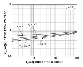
Figure 3. Base-Emitter Saturation Voltage
