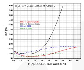
Figure 16. Inductive Load Collector Current / Voltage Crossover  $(t_c)$
