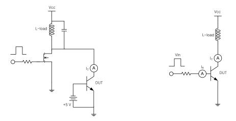
Figure 22. Energy Rating Test Circuit
