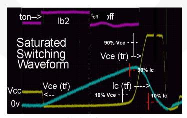
Figure 27. Saturated Switching Waveform
