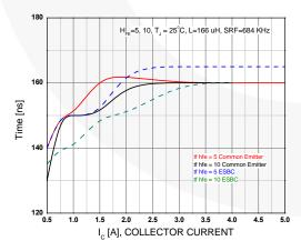
Figure 14. Inductive Load Collector Voltage Fall - Time  $(t_{\rm f})$
