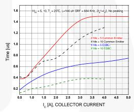
Figure 13. Inductive Load Collector Current Storage - Time (t<sub>stq</sub>)
