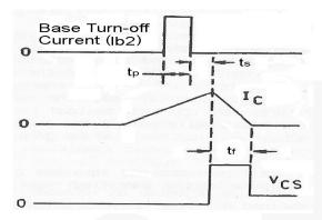
Figure 28. Storage Time - Common Emitter Base Turn Off (lb2) to I<sub>C</sub> Fall - Time
