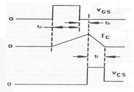
Figure 29. Storage Time - ESBC FET Gate (Off) to  $I_{\rm C}$  Fall - Time
