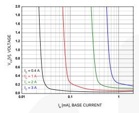
Figure 10. Typical Collector Saturation Voltage
