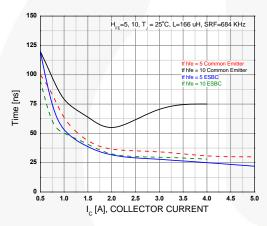
Figure 12. Inductive Load Collector Current Fall - Time  $(t_{\rm f})$
