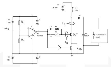
Figure 25. Simplified Saturated Switch Driver Circuit
