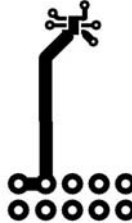
d. 151^\circ\text{C/W} when mounted on a minimum pad of 2 oz copper
